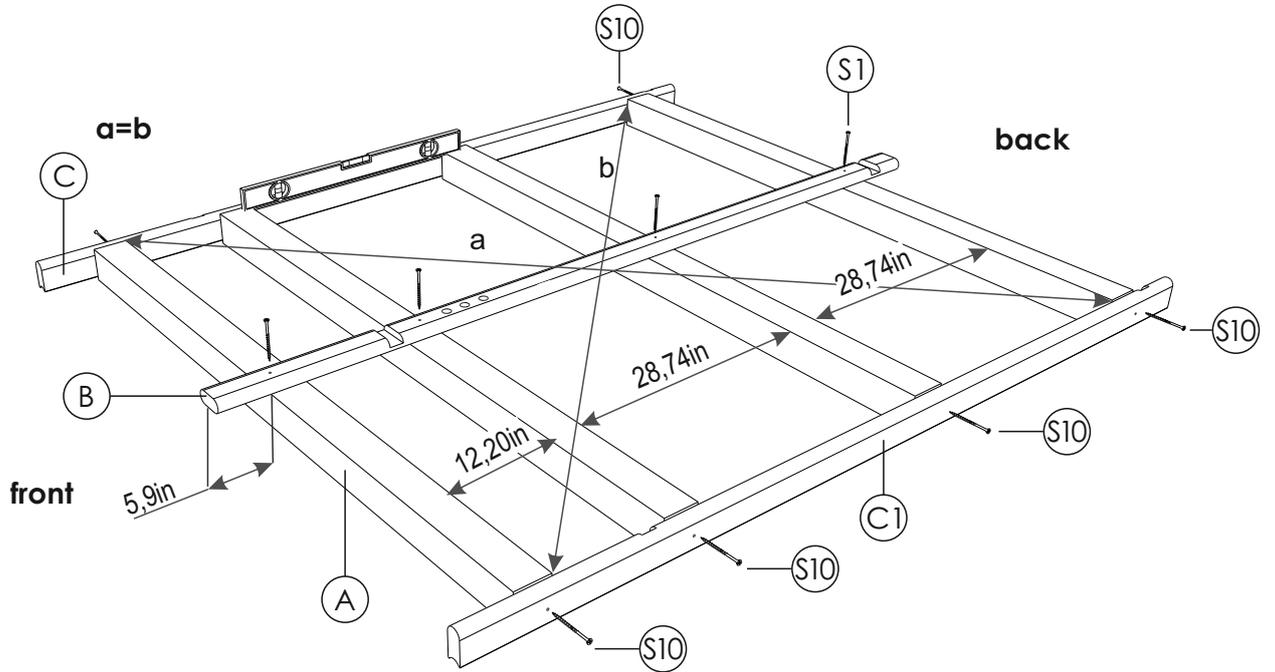
**STEP 2:** Drill 0,39in hole in each plank, in the front wall groove and in the rear wall groove to the outside. Fix 2 board panels (C2; C3) with 5x100 ss screws (S1) to each side from the centre stave. Use 8 screws for each panel as shown in picture. Between panel and stave use foam for better insulation.
