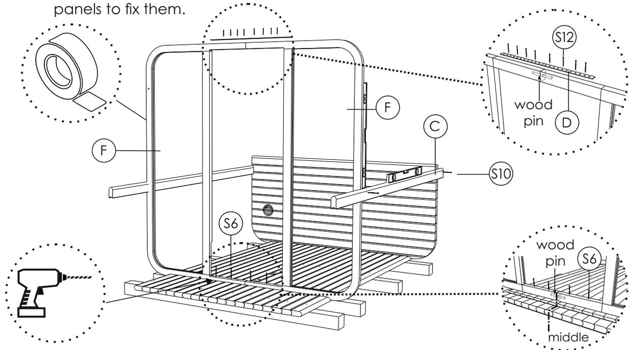
**STEP 6:** For both sides, the 10th to 11th stave (C) needs to be fixed as one piece. One is holding those three staves, and the other is fixing only the 12th; 13th; 14th; stave with screws 4x60(S10). Between floor panel and every stave use foam for better insulation.
