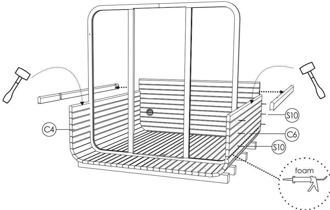
**STEP 8:** Install the panoramic panel (V1) with caution. Use foam between panels for insulation. Place it on top of the back panel. Check that side edges are aligned properly with both panels. One keeps holding the panel in line, and the other is fixing the staves (C; C1) on each sides curve using screws 4x60(S10). Check levels and fix the panel with screws at the ends of the panel's lower sides using screws 5x120(S4).
