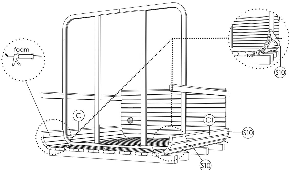
**STEP 7:** Fix the next board panels (C4; C6) on both sides with foam between the stave and panel with screws 4x60(S10) for each side. Use a rubber hammer if necessary, possibly need to push a bit back and front panels.
