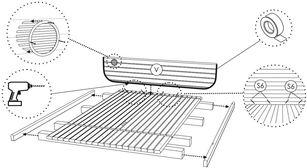
**STEP 4:** Attach adhesive tape along the rear panel (V2) edge. Pre-drill holes then fix panel V2 to panel V with two screws 5x120(S4). Between both panels use foam for better insulation.
