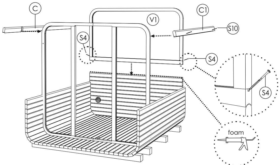
**STEP 9:** Fix the next board panels (C4; C5; C6; C7) on both sides with foam between the stave and panel with screws 4x60(S10) for each side. Use a rubber hammer if necessary, possibly need to push a bit back and front panels.
