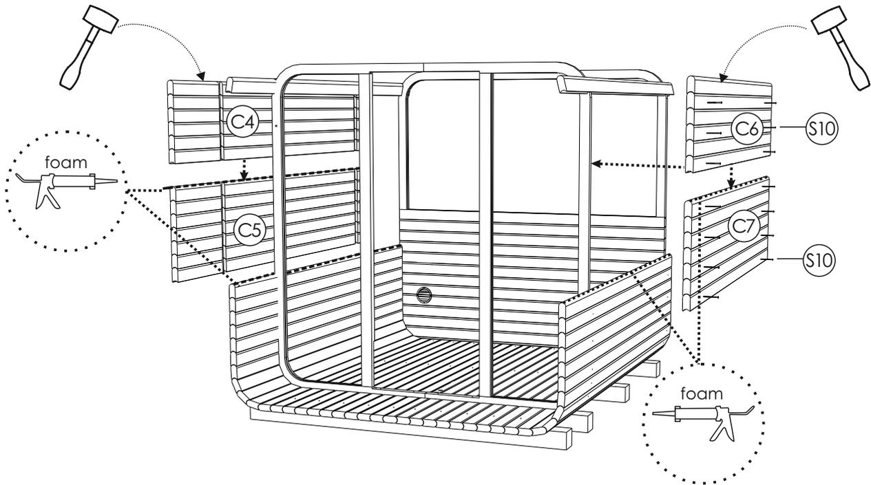
**STEP 10:** Fix the next body staves (C; C1) and board panels (C2;C3) on both sides with foam between the stave and panel with screws 4x60(S10) for each side. Use a rubber hammer if necessary, possibly need to push a bit back and front panels.
