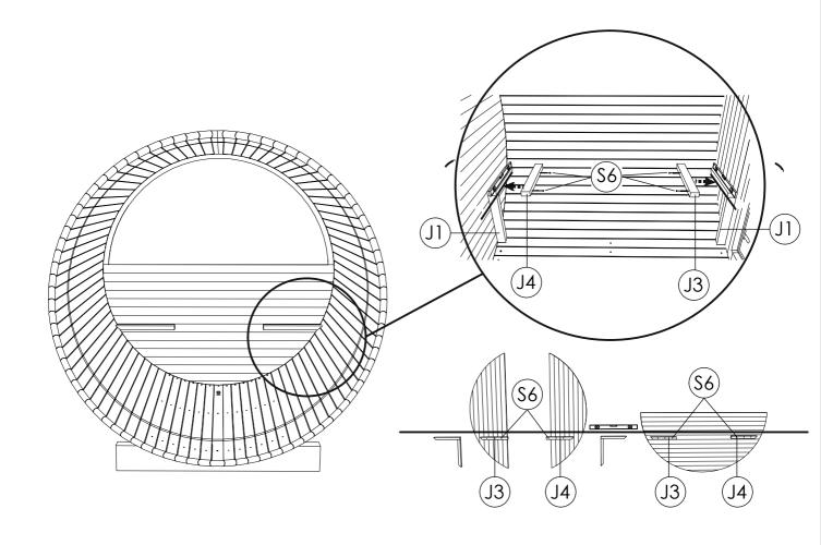
STEP 12: Install interior supporting leg (J1) in the center of bench (J). Stand bench on side wall mounts. Place J1 in the center and check the level. Using screw 5.0 x 70 SS (S6) fix bench leg to the wall and floor.
