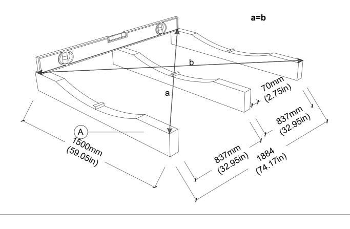
STEP 2: Place the support cradles (A) on level site. Carefully level for better stability. Place the center stave (B) on wooden dowels embedded in outer support cradles (A). Fix the center stave (B) with 5.0x100 SS(S1).
