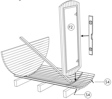
STEP 6: Attach side panel (F) using 4 5.0 x 120 (S4) screws.One person still holds door panel. Place body stave (C) on rear and front panel to connect both panels using 4.0 x 70 SS (S2) screws. Check panel level before fix them. These panels must be completely seated into the floor groove. Fix ventilation grill from inside on ventilation cuts.
