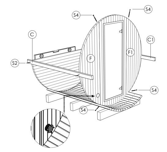
STEP 7: Attach side panel (F1) using 4 5.0 x 120 (S4) screws.One person still holds door panel. Place body stave (C) on rear and front panel to connect both panels using 4.0 x 70 SS (S2) screws. Check panel level before fixed them. These panels must be completely seated into the floor groove. Continue placing body staves (C,C1) tightly on both sides of the sauna using rubber mallet to tighten gaps.
