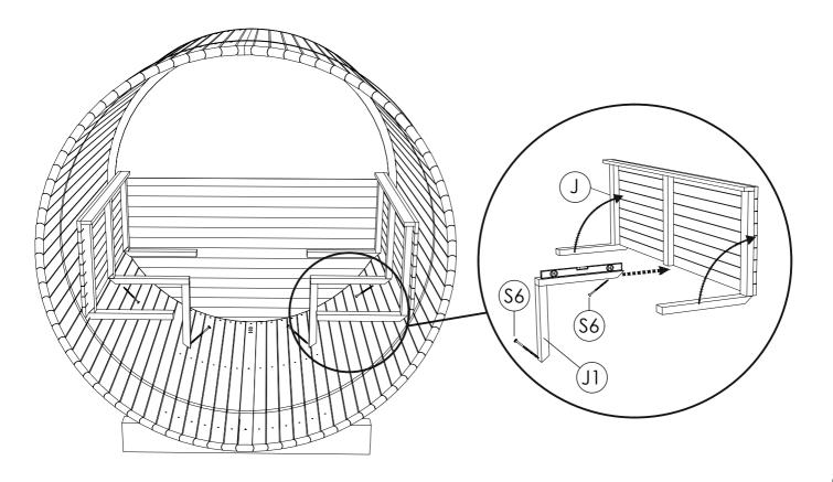
STEP 13: Install backrests (J2) at your chosen height using screw 4.0 x 50 SS (S5). Fix sauna bench (J) to wall mounts and support leg using 5 x70 SS (S6) screws.
