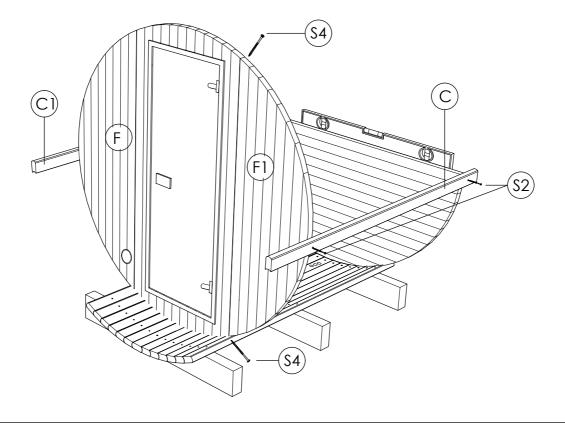
STEP 8: Place body staves (C,C1) until the halfway point on each side at the same time. Place rear panel with panoramic window (V1) on top of a rear panel (V), Fix by screw 5.0 x 120 (S4). One is holding rear panel till on both sides staves are fixed. Bind panels (F2; V1) together by temporarily placing two body staves (C) on each side fixed by screws 4.0 x 70.
