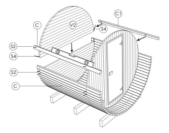
STEP 9: Continue placing body staves (C,C1) tightly on both sides of the sauna using rubber mallet, and fixing body staves with screws 4.20x70(S2). To finish the roof top joint, use roof finishing item (H). Different thickness filling peaces (H1)are provided to completely fill the gap.
