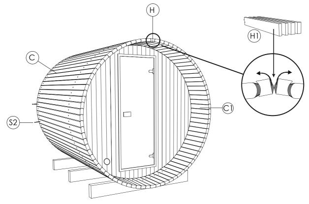
STEP 10: Install steel bands (I) by wrapping bands around barrel prior to connecting with bolts and nuts (S9). Place steel bands evenly around barrel, covering screw heads. Measure steel band to barrel edge to ensure the steel band is even all around barrel. Install interior aspen roof trim (O) with 4.0 x 50 SS (S5) screws.
