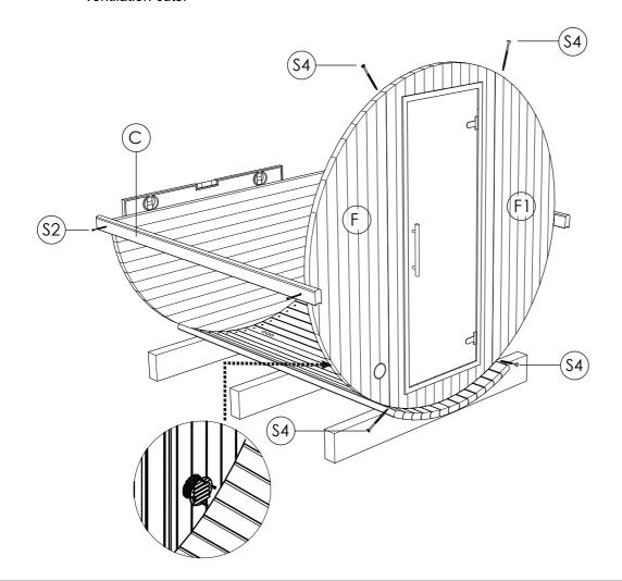
STEP 7: Firstly, position the body staves (C) until you reach the halfway point. Secondly, take the upper rear panel (V2) and place it on the bottom rear panel (V). Secure it by using 2 screws 5.0 x 120 (S4). Lastly, temporarily connect the panels (F2; V2) together by placing one or two body staves (C) on top of them.
