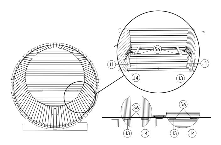
STEP 11:Install interior supporting leg (J1) in the center of bench (J). Stand bench on side wall mounts. Place J1 in the center and check the level. Using screw 5.0 x 70 SS (S6) fix bench leg to the wall and floor.
