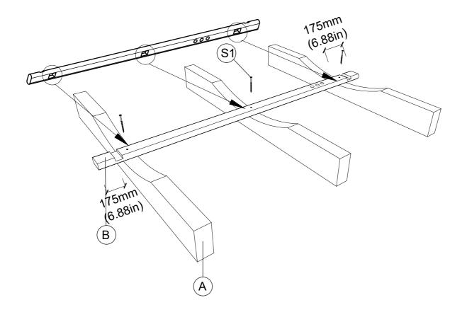
STEP 3: Place 6 sauna body staves (C) to each side of the center stave (B)and fix with screws 5.0x100 SS (S1). Be sure to align the panel groove on every next body stave, to do that use rubber hammer.
