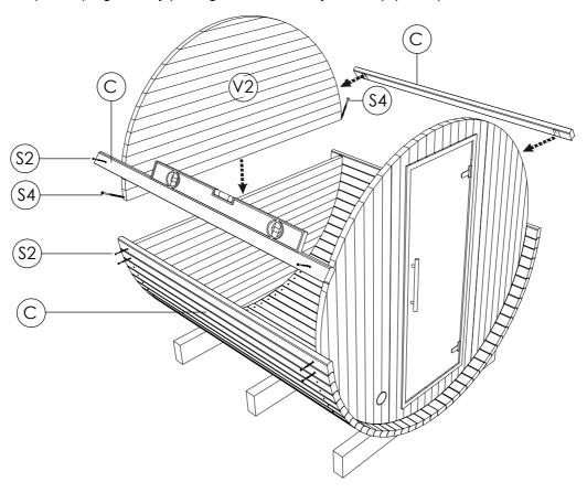
STEP 8: Continue placing body staves (C) tightly on both sides of the sauna using rubber mallet, and fixing body staves with screws 4.0x70(S2). To finish the roof top joint, use roof finishing item (H). Different thickness filling peaces (H1)are provided to completely fill the gap.
