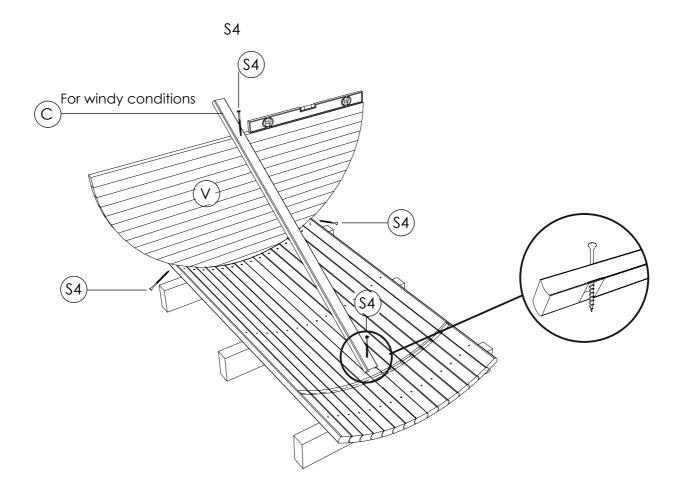
STEP 7: Attach side panel (F1) using 4 5.0 x 120 (S4) screws. One person still holds door panel. Place body stave (C) on rear and front panel to connect both panels using 4.0 x 70 SS (S2) screws. Check panel level before fixed them. These panels must be completely seated into the floor groove. Continue placing body staves (C,C1) tightly on both sides of the sauna using rubber mallet to tighten gaps.
