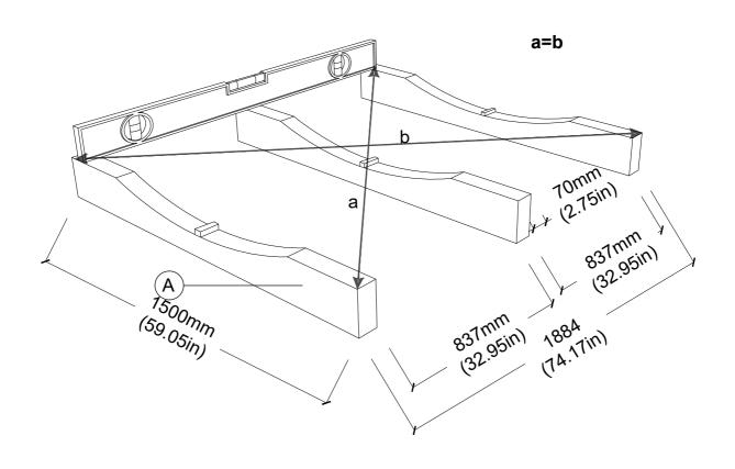
STEP 2: Place the support cradles (A)on level site. Carefully level for better stability. Place the center stave (B) on wooden dowels embedded in outer support cradles (A). Fix the center stave (B) with 5.0x100 SS(S1).
