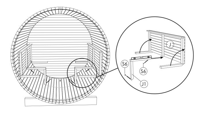
STEP 12:Install backrests (J2) at your chosen height using screw 4.0 x 50 SS (S5). Fix sauna bench (J) to wall mounts and support leg using 5 x70 SS (S6) screws.
