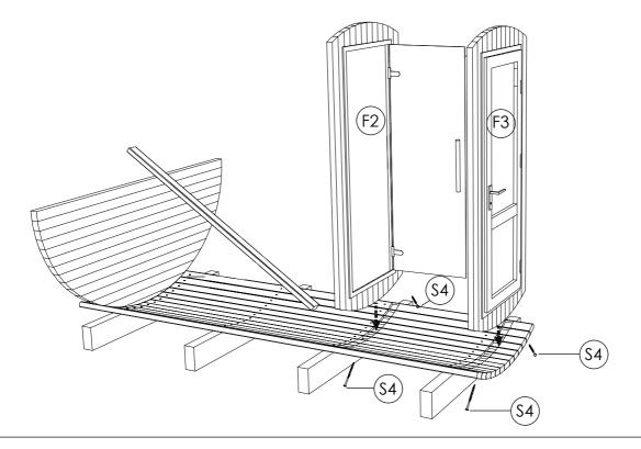
STEP 6: Attach side panel (F;F4) using four 5.0 x 120 (S4) screws.One person still holds door panel. Place body stave (C) on rear and front panel to connect both panels using 4.0 x 70 SS (S2) screws. Check panel level before fix them.These panels must be completely seated into the floor groove. Fix ventilation grill from inside on ventilation cuts.
