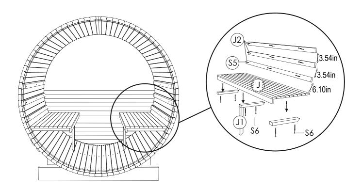
STEP 15: Install interior supporting leg (J1) in the center of bench (J). Stand bench on side wall mounts. Place J1 in the center and check the level. Using screw 5.0 x 70 SS (S6) fix bench leg to the wall and floor. Install backrests (J5) at your chosen height using screw 4.0 x 50 SS (S5). Fix sauna bench (J)to wall mounts and support leg using 5 x70 SS (S6) screws.
