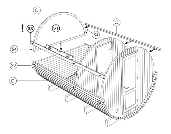
STEP 10: To complete the sauna assembly, continue to tightly place body staves (C) on both sides using a rubber mallet. Secure the body staves on the front panel with 4.20x70 screws (S2) and attach the rear window panel (V1) with 4.0 x 50 screws (S3) to prevent glass from breaking. For the rooftop joint, use the roof finishing item (H) and fill any gaps with the provided filling pieces of varying thickness (H1).
