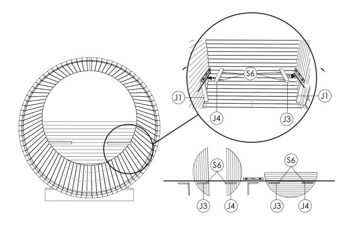
STEP13: Install interior supporting leg (J1) in the center of bench (J). Stand bench on side wall mounts. Place J1 in the center and check the level. Using screw  $5.0 \times 70$  SS (S6) fix bench leg to the wall and floor.
