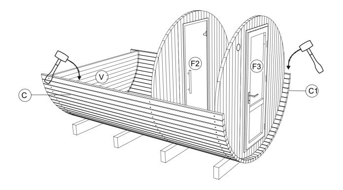
STEP 9: Place rear panel with panoramic window (V1) on bottom rear panel (V), fix by 2 screws 5.0 x 120 (S4). Bind panels (F;F2; V1)together by temporarily placing two body staves (C) on each side.
