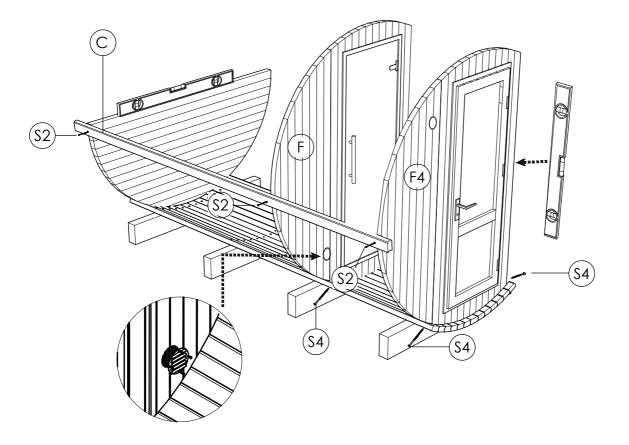
STEP 7: Attach side panel (F1;F5) using four 5.0 x 120 (S4) screws.One person still holds door panel. Place body stave (C) on rear and front panel to connect both panels using 4.0 x 70 SS (S2) screws. Check panel level before fix them. These panels must be completely seated into the floor groove. Continue placing body staves (C,C1) tightly on both sides of the sauna using rubber mallet to tighten gaps.
