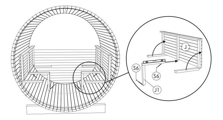
STEP 14: Install backrests (J2) at your chosen height using screw 4.0 x 50 SS (S5). Fix sauna bench (J) to wall mounts and support leg using 5 x70 SS (S6) screws.
