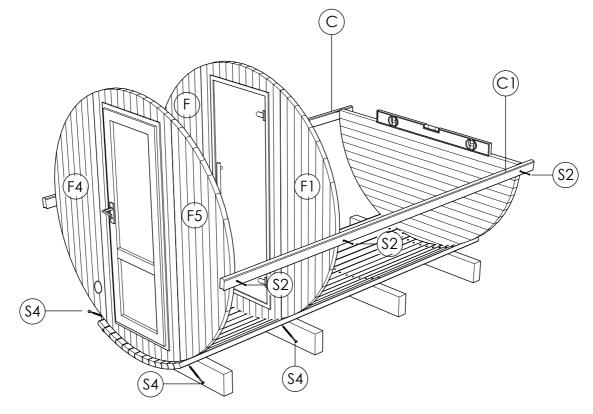
STEP 8: Place body staves (C,C1) until the halfway point on each side at the same time. Use rubber mallet to tighten gaps.
