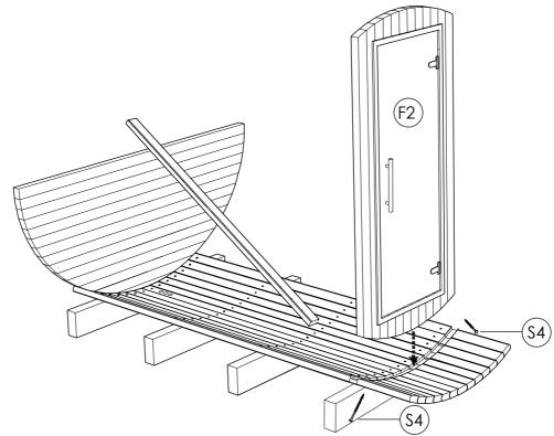
STEP 6: Attach side panel (F; F1) using 5.0 x 120 (S4) screws. One person still holds door panel. Place body stave (C) on rear and front panel to connect both panels using 4.0 x 70 SS (S2) screws. Check panel level before fix them. These panels must be completely seated into the floor groove. Fix ventilation grill from inside on ventilation cuts.
