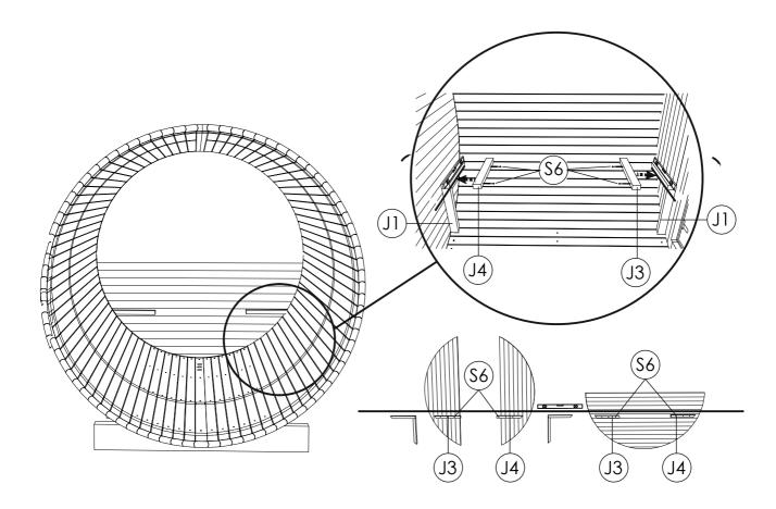
STEP 11:Install interior supporting leg (J1) in the center of bench (J). Stand bench on side wall mounts.
