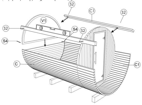
STEP 8: To complete the sauna assembly, continue to tightly place body staves (C) on both sides using a rubber mallet. Secure the body staves on the front panel with 4.20x70 screws (S2) and attach the rear window panel (V1) with 4.0 x 50 screws (S3) to prevent glass from breaking. For the rooftop joint, use the roof finishing item (H) and fill any gaps with the provided filling pieces of varying thickness (H1).
