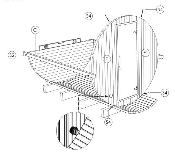
STEP 7: Put the body staves (C) in place up to the midpoint. Then, take the rear panel with the panoramic window (V1) and position it onto the bottom rear panel (V). Use two 5.0 x 120 screws (S4) to secure it. Connect the panels (F; F2; V1) by temporarily putting two body staves (C) on each side.
