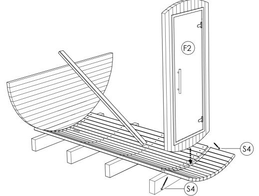
STEP 6: Attach side panel (F; F1) using 5.0 x 120 (S4) screws.One person still holds door panel. Place body stave (C) on rear and front panel to connect both panels using 4.0 x 70 SS (S2) screws. Check panel level before fix them. These panels must be completely seated into the floor groove. Fix ventilation grill from inside on ventilation cuts.
