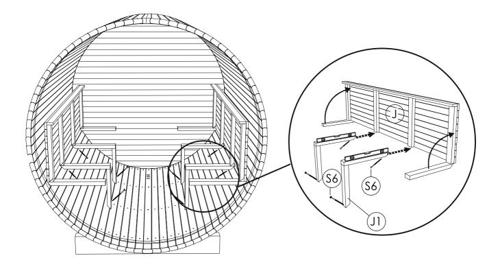
STEP 12: Install backrests (J2) at your chosen height using screw 4.0 x 50 SS (S5). Fix sauna bench (J) to wall mounts and support leg using 5 x70 SS (S6) screws.
