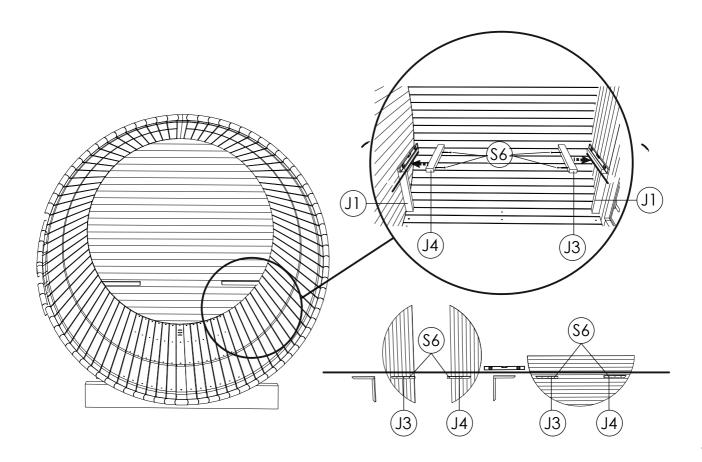
STEP11: Install interior supporting leg (J1) in the center of bench (J). Stand bench on side wall mounts. Place (J1) opposite to bench cross boards in the center and check the level. Using screw 5.0 x 70 SS (S6) fix bench leg to the wall and floor.
