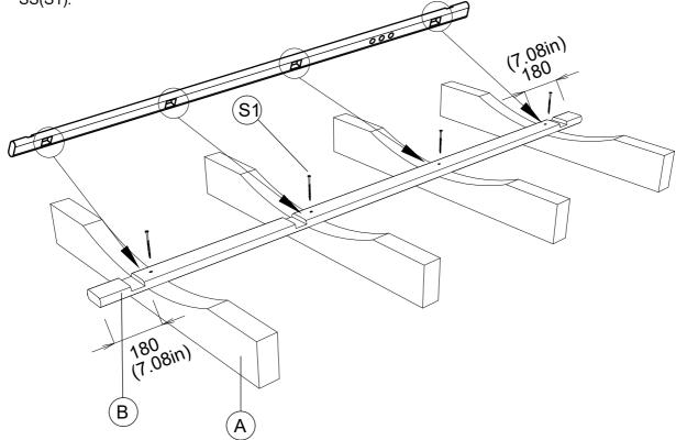
STEP 3: Place 7 sauna body staves (C) to each side of the center stave (B)and fix with screws 5.0x100 SS (S1). Be sure to align the panel groove on every next body stave, to do that use rubber hammer.
