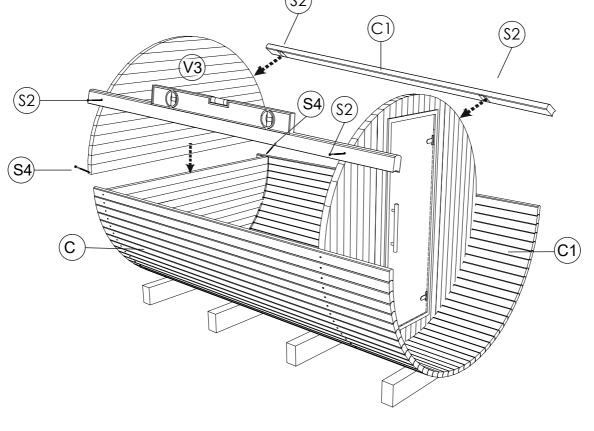
STEP 8: Continue placing body staves (C,C1) tightly on both sides of the sauna using rubber mallet, and fixing body staves with screws 4.20x70(S2). To finish the roof top joint, use roof finishing item (H). Different thickness filling peaces (H1)are provided to completely fill the gap.
