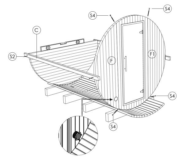
STEP 7:Place body staves (C,C1) until the halfway point on each side at the same time. Place rear panel with panoramic window (V1) on top of a rear panel (V), Fix by screw 5.0 x 120 (S4). One is holding rear panel till on both sides staves are fixed. Bind panels (F2; V1) together by temporarily placing two body staves (C)on each side fixed by screws 4.0 x 70.
