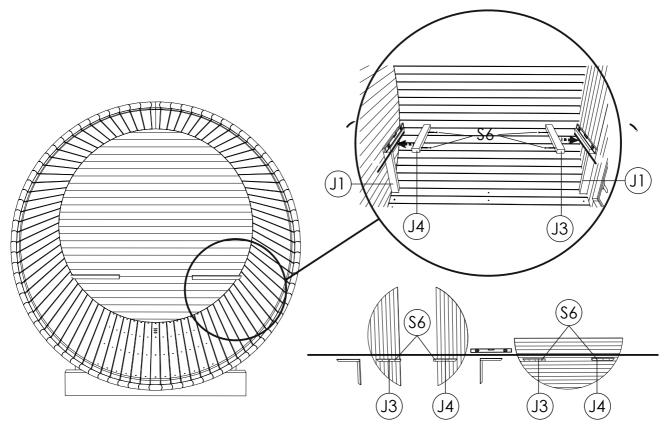
STEP 11:Install interior supporting leg (J1) in the center of bench (J). Stand bench on side wall mounts. Place J1 in the center and check the level. Using screw 5.0 x 70 SS (S6) fix bench leg to the wall and floor.
