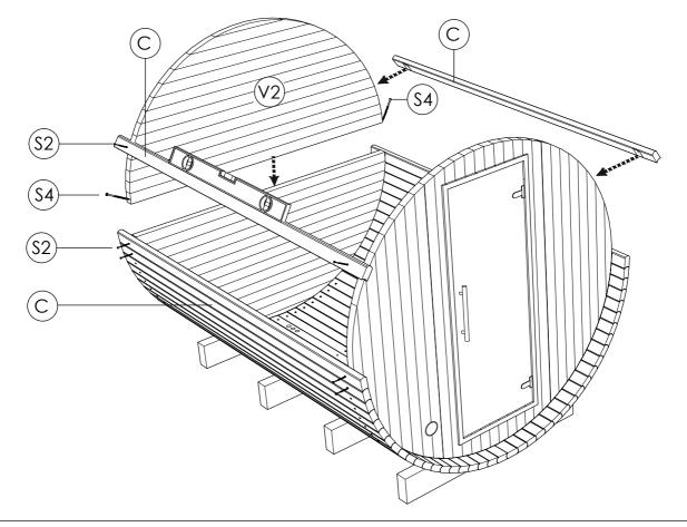
STEP 8: Continue placing body staves (C) tightly on both sides of the sauna using rubber mallet, and fixing body staves with screws 4.0x70(S2). To finish the roof top joint, use roof finishing item (H). Different thickness filling peaces (H1)are provided to completely fill the gap.
