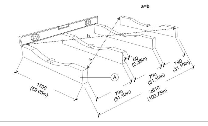
STEP 2: Place the center stave (B) on wooden dowels embedded in support cradles (A). Fix the center stave (B) with screw 5.0x100 NT(S1).
