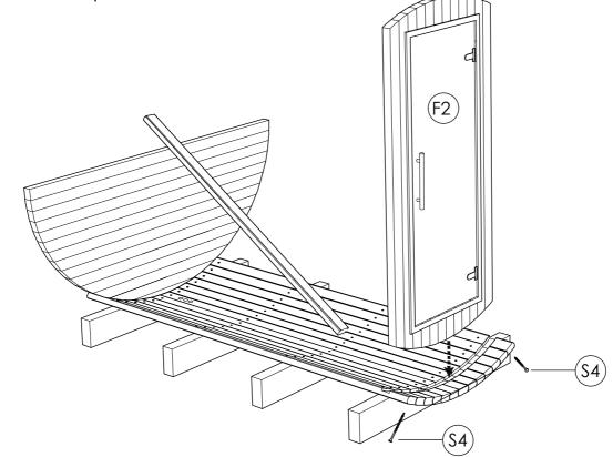
STEP 6: Attach side panel (F) using 4 5.0 x 120 (S4) screws.One person still holds door panel. Place body stave (C) on rear and front panel to connect both panels using 4.0 x 70 SS (S2) screws. Check panel level before fix them. These panels must be completely seated into the floor groove. Fix ventilation grill from inside on ventilation cuts
