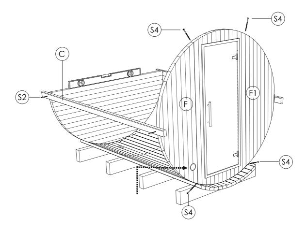
STEP 7: Place body staves (C) until the halfway point. Place upper rear panel (V2) on bottom rear panel (V), fix by 2 screws 5.0 x 120 (S4). Bind panels (F2; V2)together by temporarily placing one or two body stave (C) on top of them.
