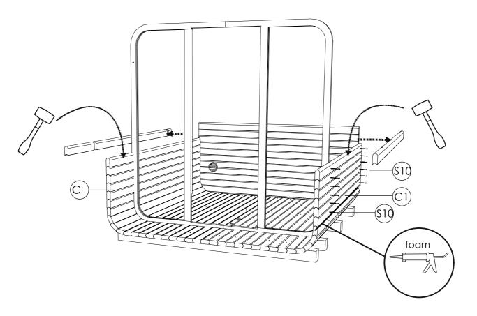
**STEP 7:** Install the upper rear panels! (V3;V4) with caution. Use foam between panels for insulation. Place it on top of the back panel. Check that side edges are aligned properly with both panels. One keeps holding the panel in line, and the other is fixing the staves (C; C1) on each sides curve using screws 4x60(S10). Check levels and fix the panel with screws at the ends of the panel's lower sides using screws 5x120(S4).
