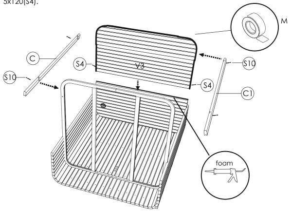
**STEP 8:** Fix the next staves (C; C1)) on both sides with foam between them with screws 4x60(S10) for each side. Use a rubber hammer if necessary.
