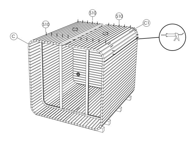
**STEP10:** If needed, use thinner staves (H1) to fill the gap between (H) staves and apply foam between staves. Install metal bands over the screw holes, then tighten the bands with screws (S9) down at the arc on one side.
