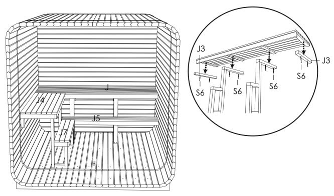
**STEP 13:**Pre-drill holes for screws. Install the ceiling board (O;O1) in the middle of the ceiling with screw 4x40SS (S11). Fix the backrest staves(J2) 5.9in up from the sauna bench. Then install backrest staves (J6) at the same height as the J2. Put in the flooring duckboard (L).
