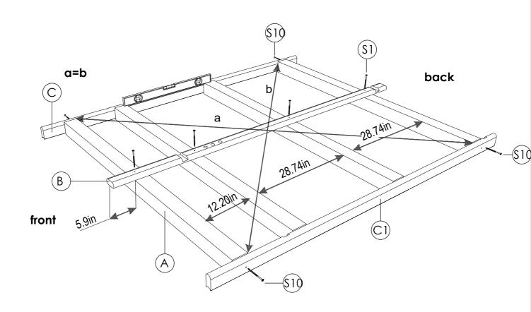
**STEP 2:** Fix 10 boards to each side(C;C1) from center board with 5x100 ss screws (S1). Between staves use foam for better insulation. Drill 10mm hole in each board, in the front wall groove and in the rear wall groove to the out-side.
