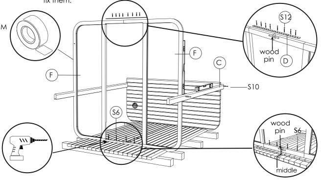
**STEP 5:**For both sides, the 11th stave (C) needs to be fixed as one piece together with 12th stave. One is holding those two staves, and the other is fixing only the 12th stave with screws 4x60(\$10). Between every stave use foam for better insulation.
