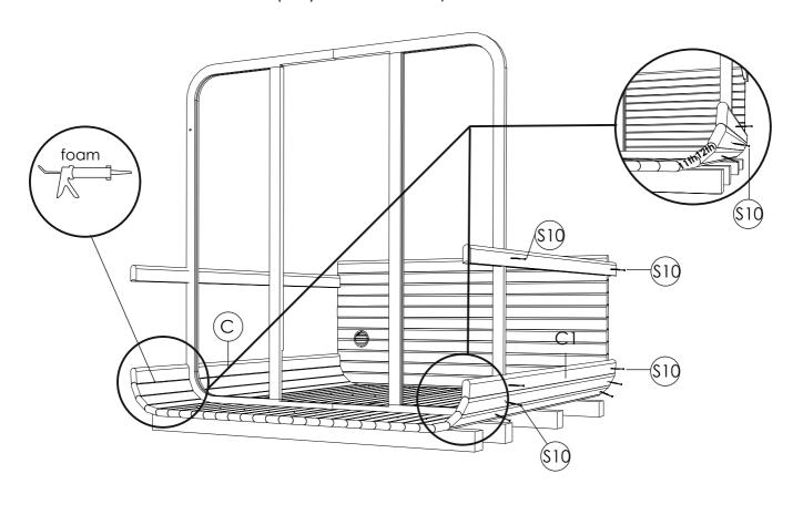
**STEP 6:**Fix the next staves (C; C1) on both sides with foam between them with screws 4x60(\$10) for each side. Use a rubber hammer if necessary.
