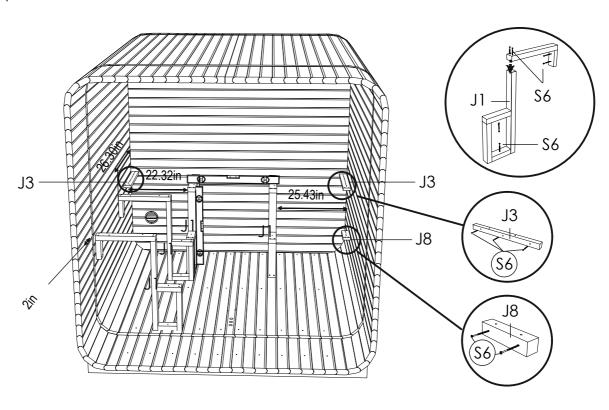
**STEP12:** Install sauna benches on top of legs (J; J7; J4; J5). Bench cross boards have to match the tops of the bench legs. Check distances from walls, then fix benches on the legs.
