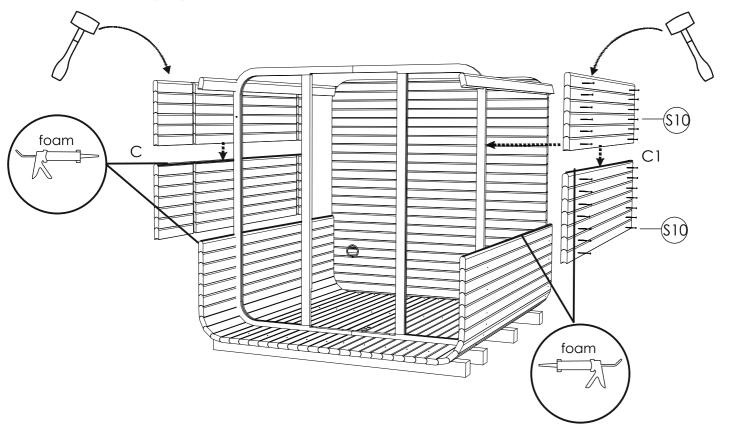
**STEP 9:** Fix the next body staves (C; C1) on both sides with foam between the staves with screws 4x60(\$10) for each side. Use a rubber hammer if necessary.
