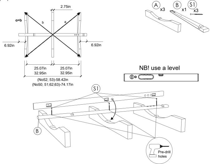
**STEP 2:** Pre-drill holes before fix staves with screws. Place 7 sauna body staves (C) to each side of the center stave (B)and fix with screws 5.0x100 SS (S1). Be sure to align the panel groove on every next body stave, to do that use rubber hammer.
