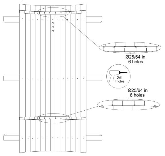
**STEP 4:** Place front bottom panel (F) in stave groove, be sure panel is centered, leveled, completely seated. Fix panel using 5.0 x 120 (S4) screws through last floor stave on both sides. NB! use a level
