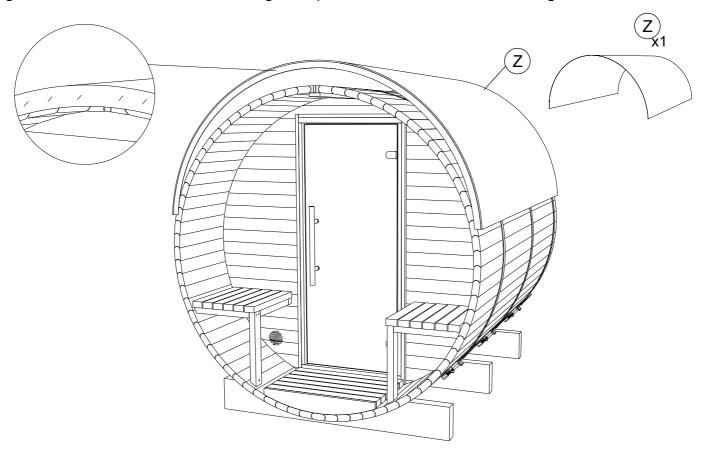
**STEP 25:** Fix with wooden slats (Z1) with screws 4.2x55 (S7) on the rain jacket bottom. The number of screws may vary depending on the sauna model.
