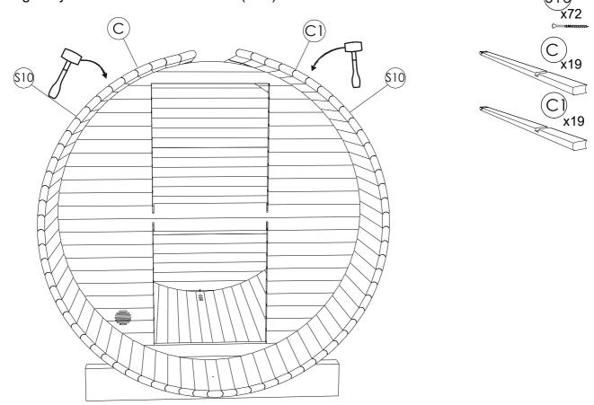
**STEP 10:** To finish the roof top joint, don't screw about last 3 boards (C) to each side, use roof finishing item (H). Different thickness filling pieces (H1) are provided to completely fill the gap. Once necessary parts are in, fix last boards with screws.
