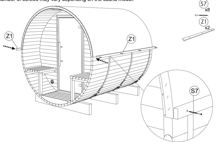
**STEP 26:** Install front and rear decorative roof finishing boards (W), fixing by screws 4.2x55(S7). Start with a center board placing it at the top of the middle of the sauna, aprox.0,7874in above roof or 0,1969in under the roof. Then fix next boards right next to previous board.
