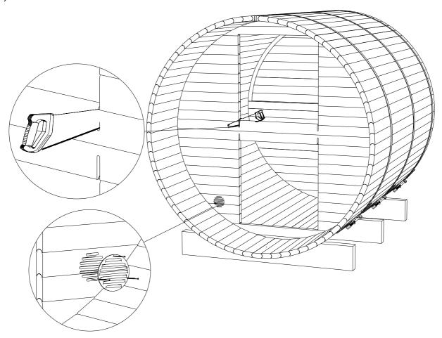
STEP 13: Pre-drill holes for screws. Fix both panels together using 5.0x120 (S4) screws.
