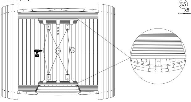
**STEP 20:** Pre-drill holes before fix with screws, install fixing blocks (L1) under floor duckboard using screw 4x50SS (S5). Place floor duckboards (L) on the floor and fix fixing blocks next to both flooring crossboards.
