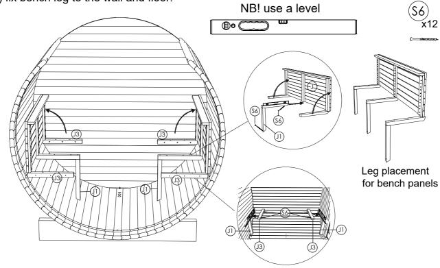
**STEP 18:** Pre-drill holes before fix backrest with screws, install backrests (J2) using screw 4.0 x 70 SS (S2). Fix sauna bench (J) to wall mounts and support leg using 5 x70 SS (S6) screws. Fix bench panel(if ordered) with screws 4.0x50SS (S5).
