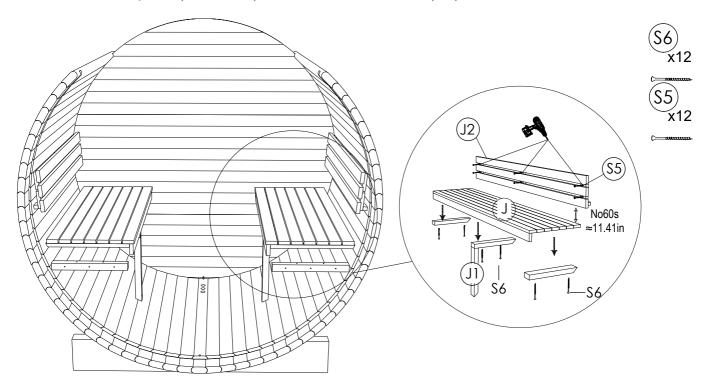
**STEP 19:** Place floor duckboards (L) to the both sides upwards and place fixing blocks next to the flooring cross boards. Pre-drill holes before fix with screws, install fixing blocks (L1) using screw or 4x50SS (S5).
