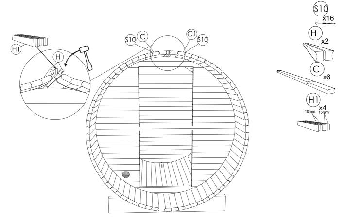
**STEP 11:** Install steel bands (I) by wrapping bands around the barrel, then connect with bolts and nuts (S9). Place steel bands evenly around the barrel approx 19.68in from terrace and 3.93in from sauna back. Bands should cover screw heads evenly. The middle band should be evenly placed from both bands. The bands should be tense, they cant be loosened.
