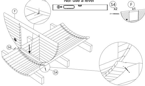
**STEP 5:** Place rear panel (V) in stave groove, be sure panel is centered, leveled, completely seated. Fix panel using 5.0 x 120 (S4) screws through last floor stave on both sides.
