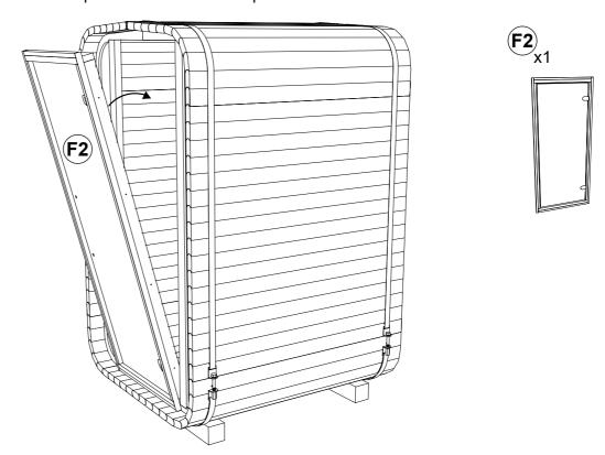
**STEP 17:** Put plastic spacers in the gap between the door box and the front panel where the screws go. Combine spacers for best width. Spacer must fit tightly.
