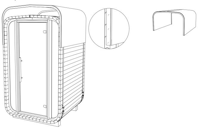
**STEP 28:** Pre-drill holes for screws. Fix wooden slats (Z1) with screws (S7) on the rain jacket bottom.
