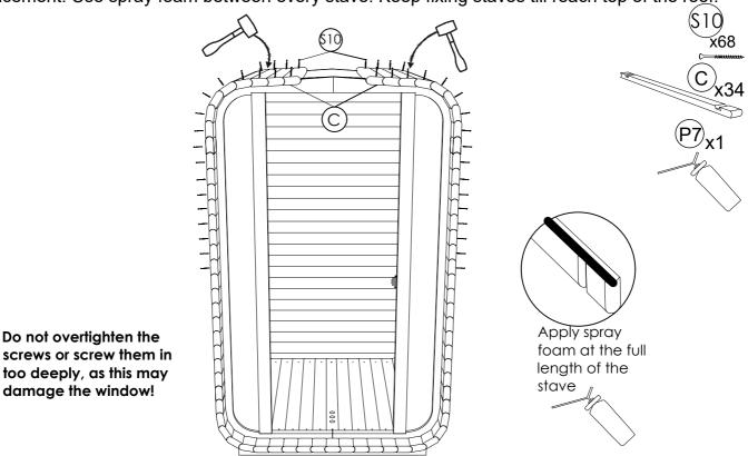
**STEP 13**: Finish roof with (C) staves and final staves (H). If needed, use thinner staves (H1) to fil the gap between (H) staves and apply spray foam between staves. Make sure that centre of the roof is tightly filled, then fix with screws (S10). It's possible that at the roof center wont be place for (H) staves and it finishes with just (C) boards.
