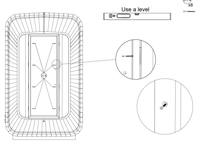
**STEP 19:** Use spray foam around door box. Let the spray foam dry. The excess amount will come off easily if you don't touch it while it's wet. Fix door moldings to both sides and on top of the door with (S5) screws.
