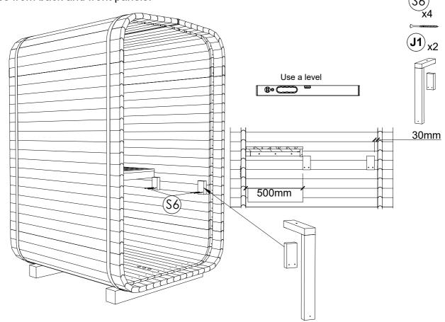
STEP 24: Fix bigger part from (J1) on fixed bench supports with (S6) screws as shown.
