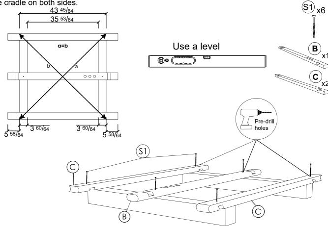
**STEP 2:** Attach five staves (C) on each side of the center stave. Check the level while installing the staves and use a rubber hammer for a tighter fit. Pre-drill holes for the screws. After fixing eight staves, remove the side staves and reattach them.
