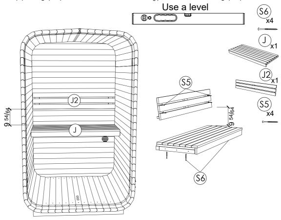
**STEP 22**: Bench leg comes in two parts. start with bigger one. Put bench leg(J1) on the side wall and draw a line, under leg upper part, for wall mount.
