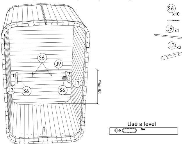
STEP 21:Fix bench (J) using (S6) screws. Fix backrest 9 <sup>54</sup>/<sub>64</sub>above bench using (S5) screws.
