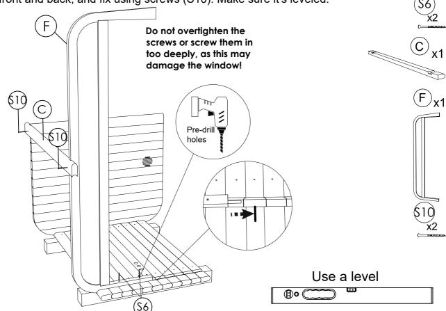
**STEP 8**: Place the second front panel (F). Slide it together that the top and bottom connects. Fix it at the panel threshold with screws (S6) pre-drill holes. Make sure it's level. Use metal bracket are to part to
