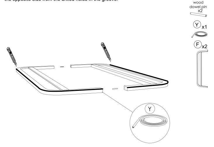
**STEP 7**: Draw a line on the center stave where the middle is. Take one of the panels (F) and put it directly next to the middle line. Fix it at the panel threshold with screws (S6). Pre-drill holes in the panel threshold, evenly spaced and not too close to the sides. Connect both panels with (C) stave, front and back, and fix using screws (S10). Make sure it's leveled.
