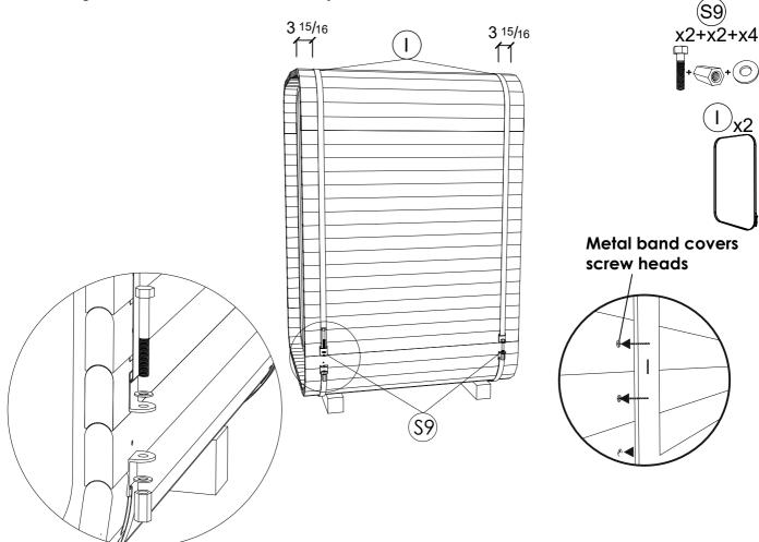
**STEP 16**:Install the doors (F2). Put the doors on threshold and lay in frame about in the middle. Fix the doors with clamps, or have another person hold the door in place.
