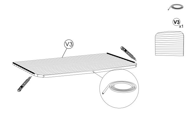
STEP 11:Install the panel (V3) with caution. Use spray foam between panels for better insulation. Place it on top of the lower back panel (V). Check level and that side edges are aligned with bottom panel. One keeps holding the panel, and the other is fixing the side stave on a upper curve using screws (S10). Secure the panel (V3) at the both corners using two screws (S4).
