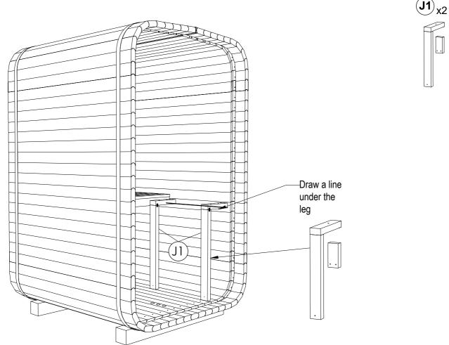
**STEP 23**: Fix smaller part from (J1) on marked line using (S6) screws. Measure necessary distances from back and front panels.
