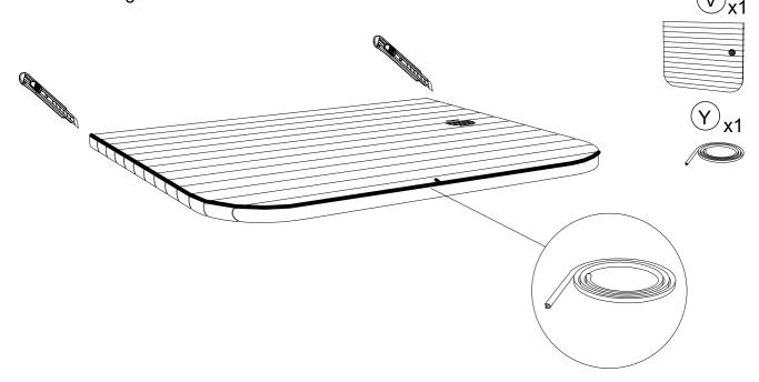
**STEP 5**:Place the rear bottom panel (V) into the board groove. Ensure the panel is level. Secure it with screws (S4) at both corners through the stave.
