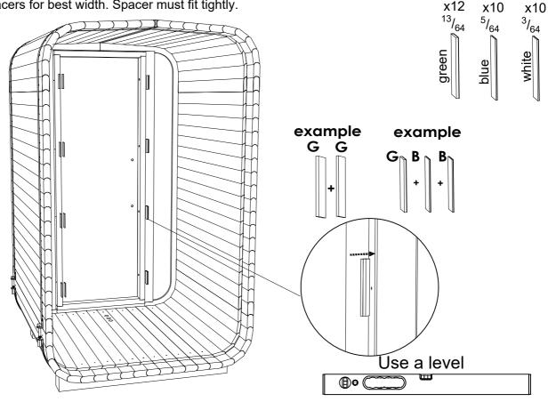
**STEP 18:** Fix one side of the door box with screws (S14) slightly to the outside through spacers. Then put spacers in other side. Combine spacers for necessary width. Spacers must fit tightly, they can't slip down before door is fixed with screws. Use screws (S14) to fix doors. Check door box, both sides should be straight, they must not be bent inwards or outwards.
