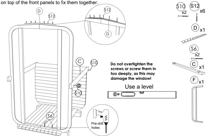
**STEP 9**: Fix 14 staves (C) on both sides with screws (S10). Use rubber hammer for tighter placement. Use spray foam between every stave. Keep fixing staves till reach top of the rear panel (V).
