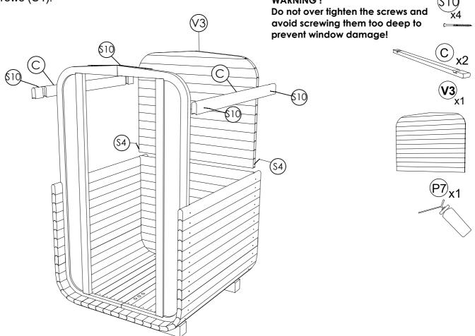
**STEP 12**: Fix 17 staves (C) on both sides with screws (S10). Use rubber hammer for tighter placement. Use spray foam between every stave. Keep fixing staves till reach top of the roof.
