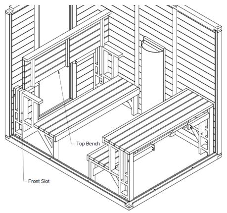
SLIDE THE BOTTOM BENCH INTO THE REAR SLOT. THEN REPEAT ON OTHER SIDE.
