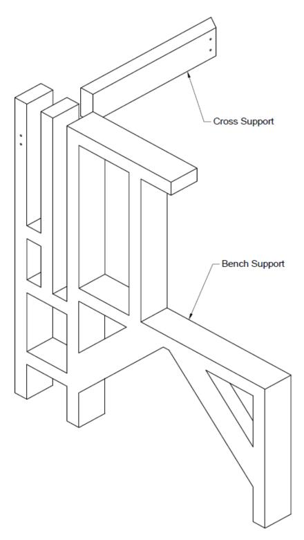
SCREW THE TWO 5" SCREWS THROUGH THE BENCH SUPPORT INTO THE CROSS SUPPORT USING THE T25 TORX BIT. MAKE SURE THE CROSS SUPPORT HAS THE ANGLE FACING THE FRONT OF THE SUPPORT. DO THIS FOR EACH BENCH SUPPORT.
