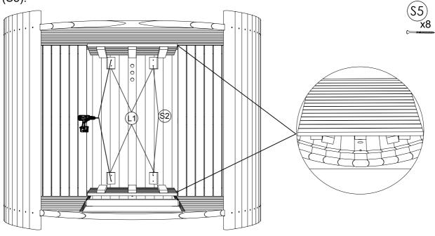
**STEP 20:** Pre-drill holes before fix with screws, install fixing blocks (L1) under floor duckboard using screw (S5). Place floor duckboards (L) on the floor and fix fixing blocks next to both flooring crossboards.
