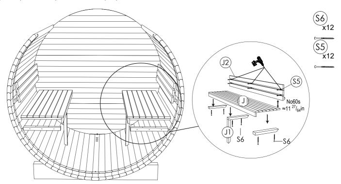
**STEP 19:** Place floor duckboards (L) to the both sides upwards and place fixing blocks next to the flooring cross boards. Pre-drill holes before fix with screws, install fixing blocks (L1) using screw or (S5).
