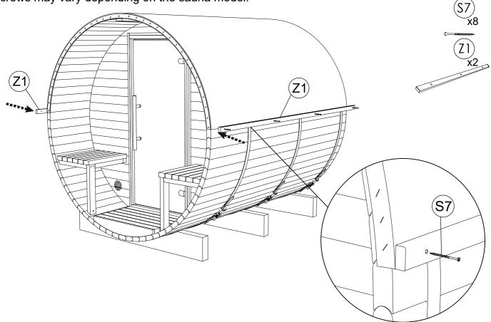
**STEP 26:** Install front and rear decorative roof finishing boards (W), fixing by screws (S7). Start with a center board placing it at the top of the middle of the sauna, aprox. $^{50}/_{64}$ in under the roof. Then fix next boards right next to previous board.
