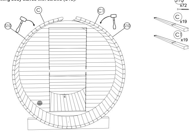
**STEP 10:** To finish the roof top joint, don't screw about last 3 boards (C) to each side, use roof finishing item (H). Different thickness filling pieces (H1) are provided to completely fill the gap. Once necessary parts are in, fix last boards with screws.
