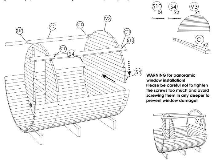
**STEP 9:** Continue placing body staves (C) tightly on both sides of the sauna using rubber mallet, and fixing body staves with screws (S10).
