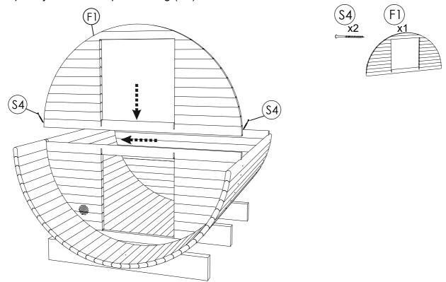
**STEP 8:** Take the upper rear panel (V3 or V1-panoramic window) and place it on the bottom rear panel (V). Secure it by using 2 screws (S4). Connect the panels (F2; V3) together by placing one body staves (C) both sides where you can reach, with (S10) screws.
