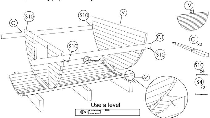
**STEP 6:** Continue placing body staves (C) tightly on both sides of the sauna using rubber mallet, and fixing body staves with screws (S10). Fix one stave higher on left side than at right.
