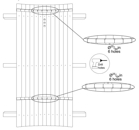
**STEP 4:** Place front bottom panel (F) in stave groove, be sure panel is centered, leveled, completely seated. Fix panel using (S4) screws through last floor stave on both sides.
