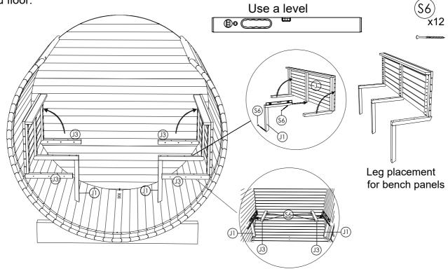
**STEP 18:** Pre-drill holes before fix backrest with screws, install backrests (J2) using screw (S2). Fix sauna bench (J) to wall mounts and support leg using (S6) screws. Fix bench panel(if ordered) with screws (S5).
