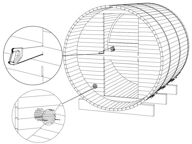
STEP 13: Pre-drill holes for screws. Fix both panels together using (S4) screws.
