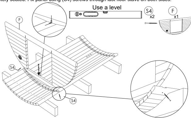
**STEP 5:** Place rear panel (V) in stave groove, be sure panel is centered, leveled, completely seated. Fix panel using (S4) screws through last floor stave on both sides.
