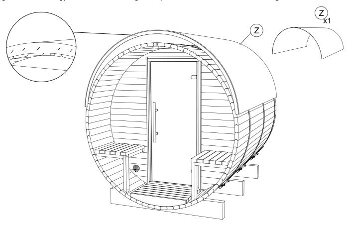
**STEP 25:** Fix wooden slats (Z1) with screws (S7) on the rain jacket bottom. The number of screws may vary depending on the sauna model.
