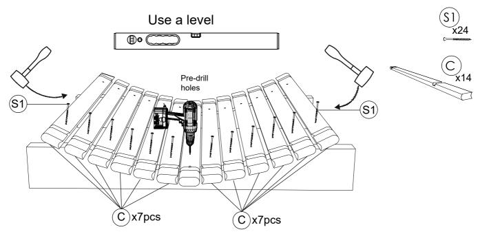
**STEP3:** Drill six  $^{25}/_{64}$ in holes in front and back wall groove to the out-side in board connections as shown in the picture.
