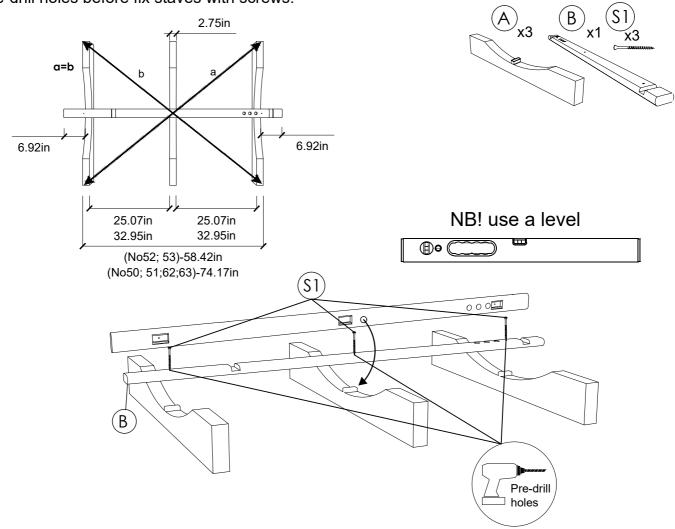
**STEP 2:** Pre-drill holes before fix staves with screws. Place 7 sauna body staves (C) to each side of the center stave (B)and fix with screws (S1). Be sure to align the panel groove on every next body stave, to do that use rubber hammer.
