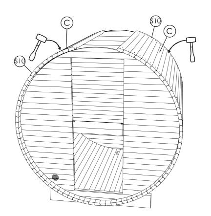
**STEP 10:** To finish the roof top joint, don't screw about last 2-3 boards (C) to each side, use roof finishing item (H). Different thickness filling pieces (H1) are provided to completely fill the gap. Once necessary parts are in, fix last boards with screws.
