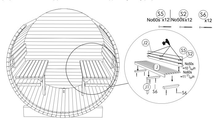
**STEP 19:** Place floor duckboards (L) to the both sides upwards and place fixing blocks next to the flooring cross boards. Pre-drill holes before fix with screws, install fixing blocks (L1) using screw(S2)No50s or (S5)No60s.
