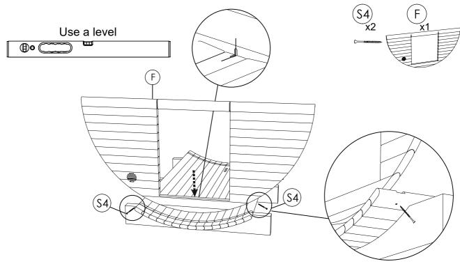
**STEP 5:** Place rear panel (V) in stave groove, be sure panel is centered, leveled, completely seated. Fix panel using (S4) screws through last floor stave on both sides. For full panoramic instruction go to 5.1 page.
