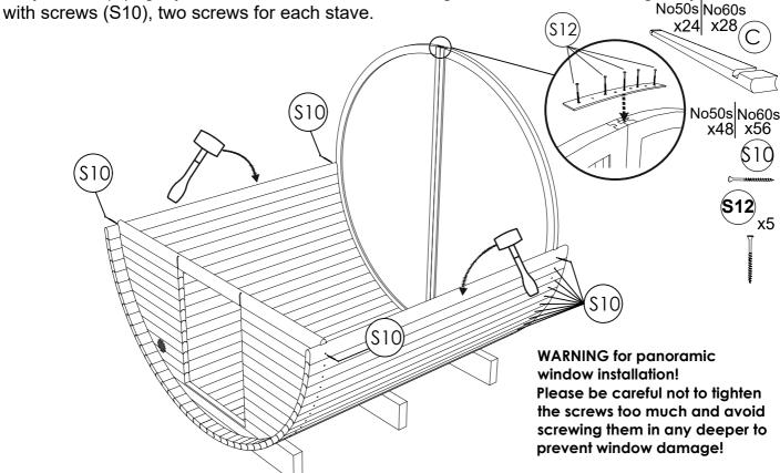
**STEP 6:** Take the upper front panel (F1) and place it on top of the front panel (F). Secure it by using 2 screws (S4). Connect the panels (F1; V1) together by placing one body stave (C) on both sides where you can reach, with (S10) screws.
