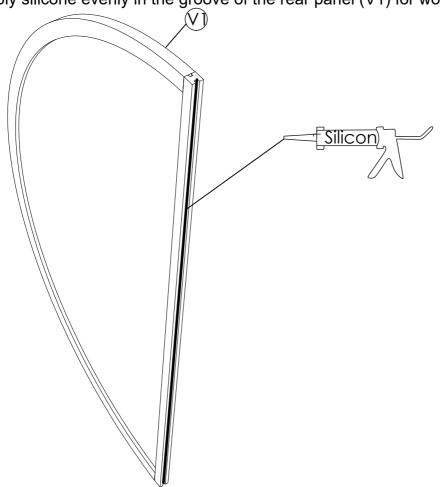
**STEP 2:** Place rear panel (V1) in stave groove, be sure panel is centered, leveled, completely seated. Fix panel using (S10) screw through last floor stave. Connect the panels (F; V1) together with body stave (C) with (S10) screw.
