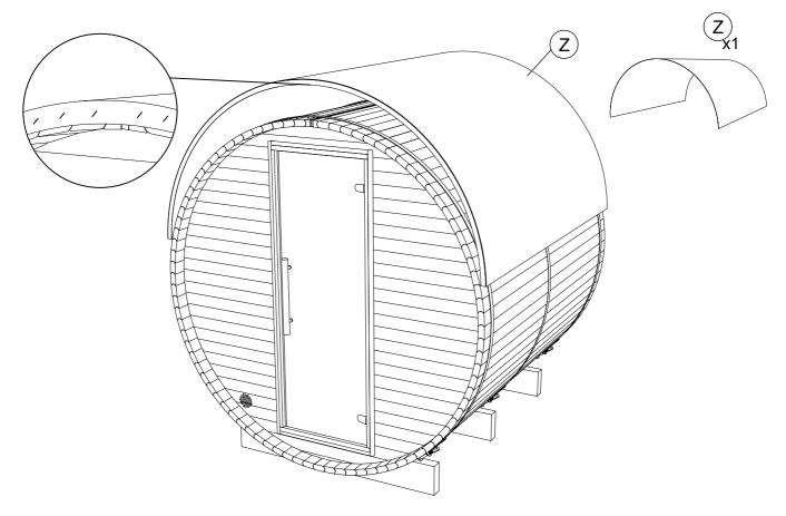
**STEP 23:** Fix with wooden slats (Z1) with screws (S7) on the rain jacket bottom. The number of screws may vary depending on the sauna model.
