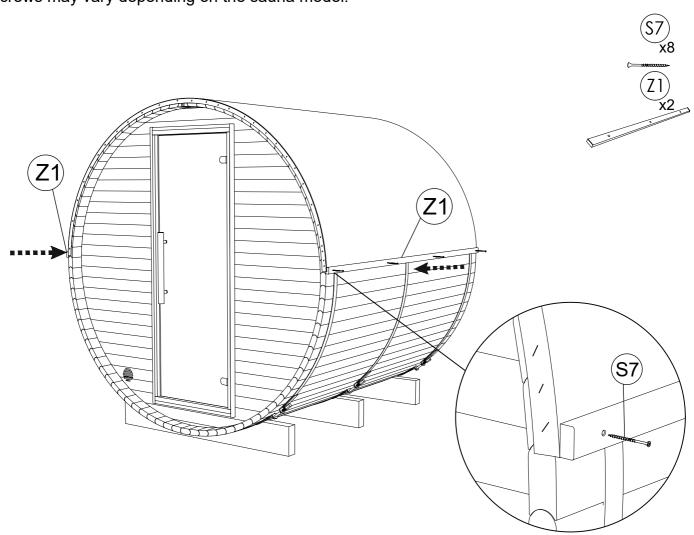
**STEP 24:** Install front and rear decorative roof finishing boards (W), fixing by screws (S7). Start with a center board placing it at the top of the middle of the sauna, aprox.  $^{50}/_{64}$  in above roof or  $^{13}/_{64}$  in under the roof. Then fix next boards right next to previous board.
