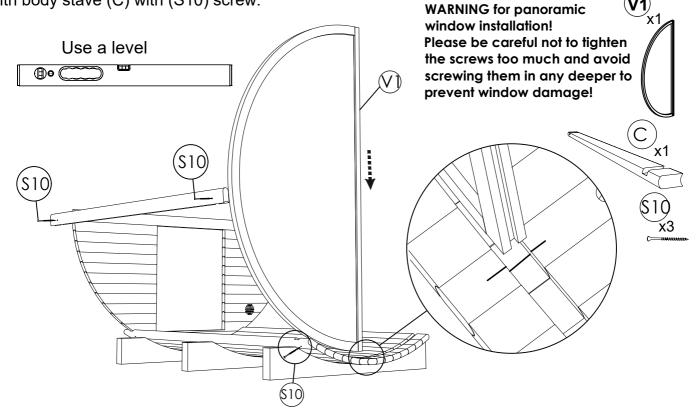
**STEP 3:** Insert wood spacer bar (V1-F) in to the fixed rear panel (V1).
