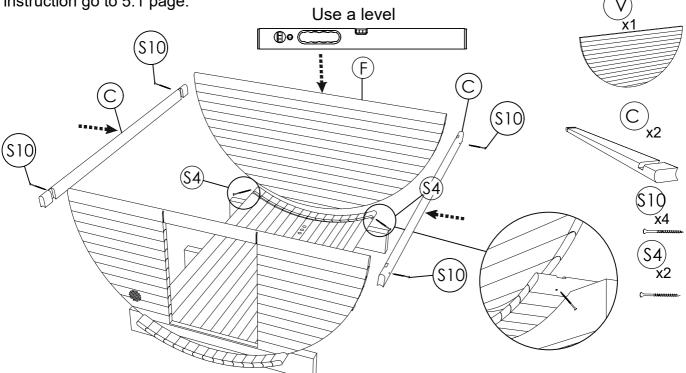
**STEP 6:** Continue placing body staves (C) tightly on both sides of the sauna using rubber mallet, and fixing body staves with screws (S10). Fix one stave higher on left side than at right.
