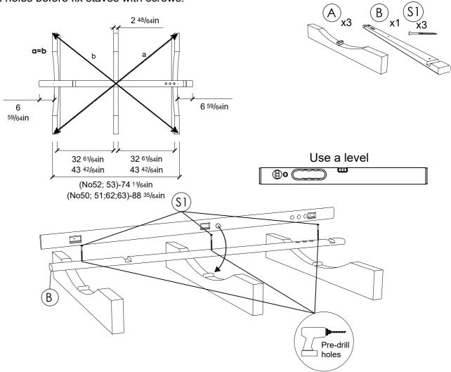
**STEP 2:** Pre-drill holes before fix staves with screws. Place 6 (No50s) or 7 (No60s) sauna body staves (C) to each side of the center stave (B)and fix with screws (S1). Be sure to align the panel groove on every next body stave, to do that use rubber hammer.
