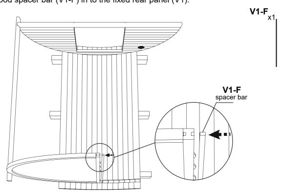
**STEP 4:** Apply silicone evenly in the groove of the second rear panel (V1). Place second rear panel (V1) in stave groove, be sure panel is centered, leveled, completely seated. Fix panel using (S10) screw through last floor stave. Connect the panels (F; V1) together with body stave (C) with (S10) screw.
