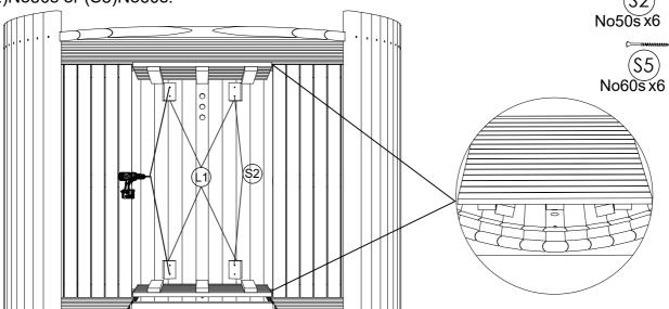
**STEP 20:** Pre-drill holes before fix with screws, install fixing blocks (L1) under floor duckboard using screw (S2) No50s or (S5) No60s. Place floor duckboards (L) on the floor and fix fixing blocks next to both flooring crossboards.
