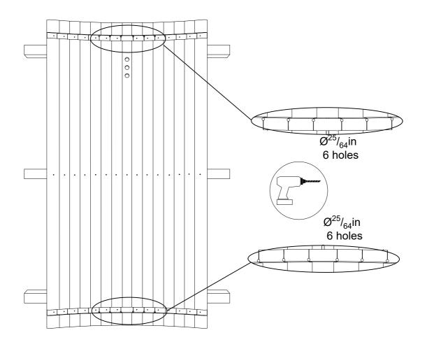
**STEP 4:** Place front bottom panel (F) in stave groove, be sure panel is centered, leveled, completely seated. Fix panel using (S4) screws through last floor stave on both sides.
