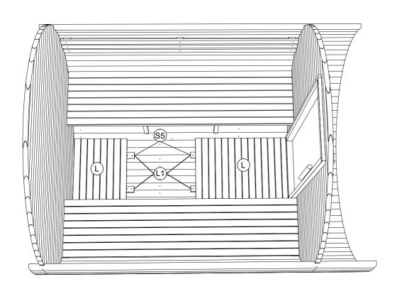
STEP 21: Place last floor duckboard (L) between both floors.
