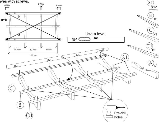
**STEP 2:** Pre-drill holes before fix staves with screws. Place 6 (R190) or 7 (No60s) sauna body staves (C) to each side of the center stave (B)and fix with screws 5.0x100 SS (S1). Be sure to align the panel groove on every next body stave, to do that use rubber hammer. Take of last board from both sides and fix it.
