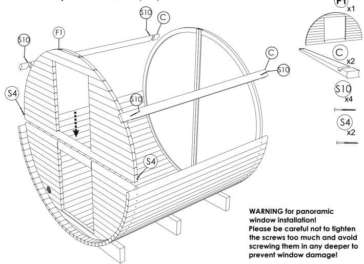
**STEP 7:** Place front top panel (F1) on front bottom panel (F), be sure panel is centered, leveled, completely seated. Fix panel using (S4) screws on both sides.
