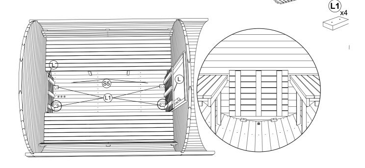
STEP 20: Pre-drill holes before fix with screws, install fixing blocks (L1) under floor duckboard using screw (S5) Place floor duckboards (L) on the floor and fix fixing blocks next to both flooring crossboards.
