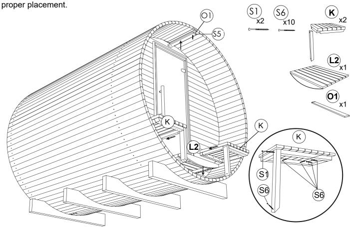
**STEP 24**: Place waterproof PVC roof cover . Align roof cover equally to both sides. Roof cover goes about 1  $^{37}/_{64}$ in over each sides edge. Staple roof cover on the saunas edge.
