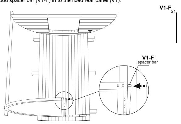
**STEP 4:** Apply silicone evenly in the groove of the second rear panel (V1). Place second rear panel (V1) in stave groove, be sure panel is centered, leveled, completely seated. Fix panel using (S10) screw through last floor stave. Connect the panels (F; V1) together with body stave (C) with (S10) screw.
