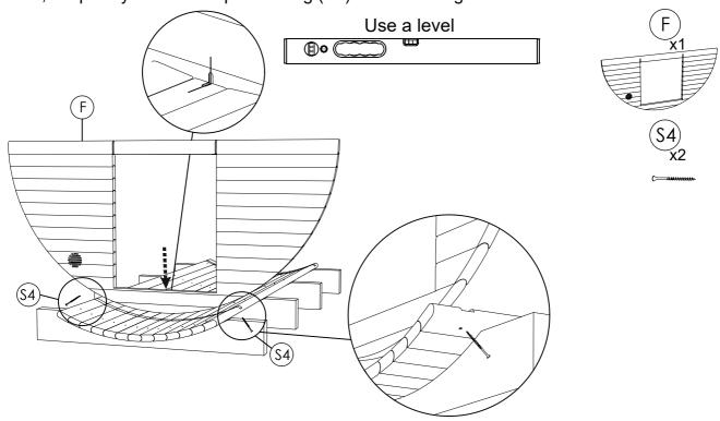
**STEP 5:** Place rear panel (V) in stave groove, be sure panel is centered, leveled, completely seated. Fix panel using (S4) screws through last floor stave on both sides. Connect the panels (F; V) together by placing one body stave (C; C1) both sides in level, with (S10) screws. For full panoramic window installation go to 5.1 page.
