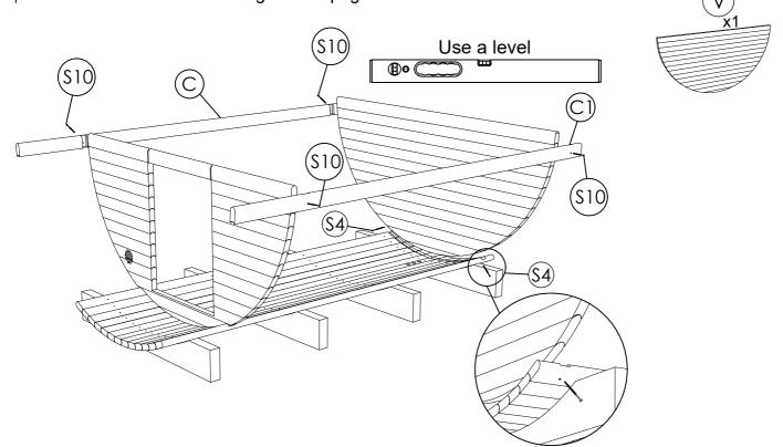
**STEP 6:** Continue placing body staves (C;C1) tightly on both sides of the sauna using rubber mallet, and fixing body staves with screws (S10).
