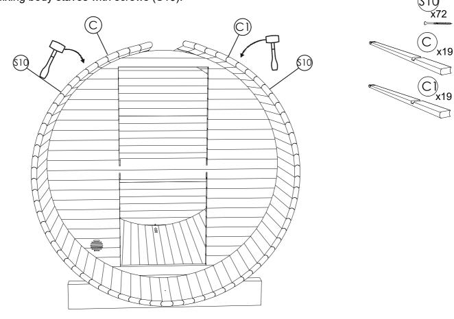
**STEP 10:** To finish the roof top joint, don't screw about last 3 boards (C) to each side, use roof finishing item (H). Different thickness filling pieces (H1) are provided to completely fill the gap. Once necessary parts are in, fix last boards with screws (S10).
