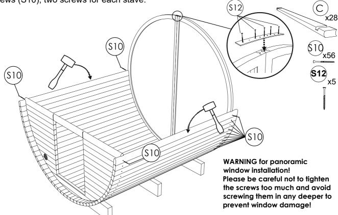
**STEP 6:** Take the upper front panel (F1) and place it on top of the front panel (F). Secure it by using 2 screws (S4). Connect the panels (F1; V1) together by placing one body stave (C) on both sides where you can reach, with (S10) screws.
