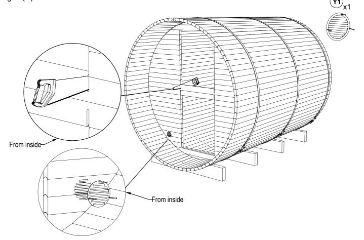
STEP 13: Pre-drill holes for screws. Fix both panels together using (S4) screws.
