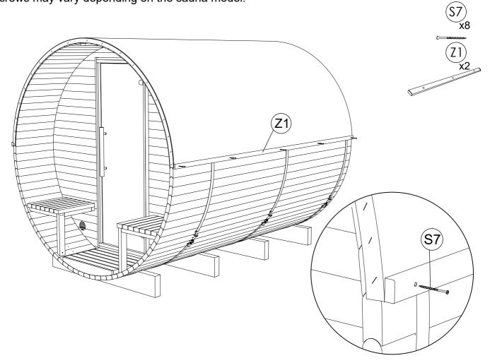
**STEP 26:** Install front and rear decorative roof finishing boards (W), fixing by screws (S7). Start with a center board placing it at the top of the middle of the sauna, aprox.  $^{50}/_{64}$  in above roof or  $^{13}/_{64}$  in under the roof. Then fix next boards right next to previous board.
