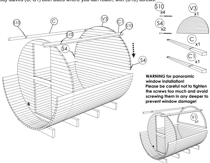
**STEP 9:** Continue placing body staves (C) tightly on both sides of the sauna using rubber mallet, and fixing body staves with screws (S10).
