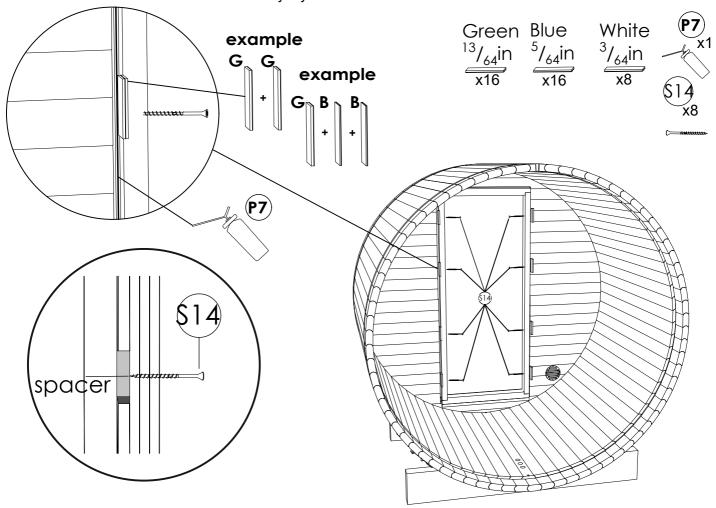
STEP 16: Fix door moldings to both sides and on top of the door with S5 screws.
