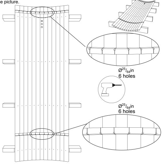
**STEP 4:** Place front bottom panel (F) in stave groove, be sure panel is centered, leveled, completely seated. Fix panel using (S4) screws through last floor stave on both sides.
