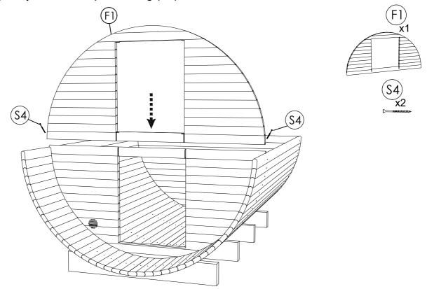
**STEP 8:** Take the upper rear panel (V3 or V1-panoramic window) and place it on the bottom rear panel (V). Secure it by using 2 screws (S4). Connect the panels (F2; V3) together by placing one body staves (C; C1) both sides where you can reach, with (S10) screws.
