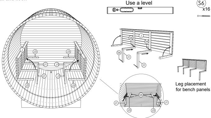
**STEP 18:** Pre-drill holes before fix backrest with screws, install backrests (J2) using screw (S2). Fix sauna bench (J) to wall mounts and support leg using (S6) screws. Fix bench panel(if ordered) with screws (S5).
