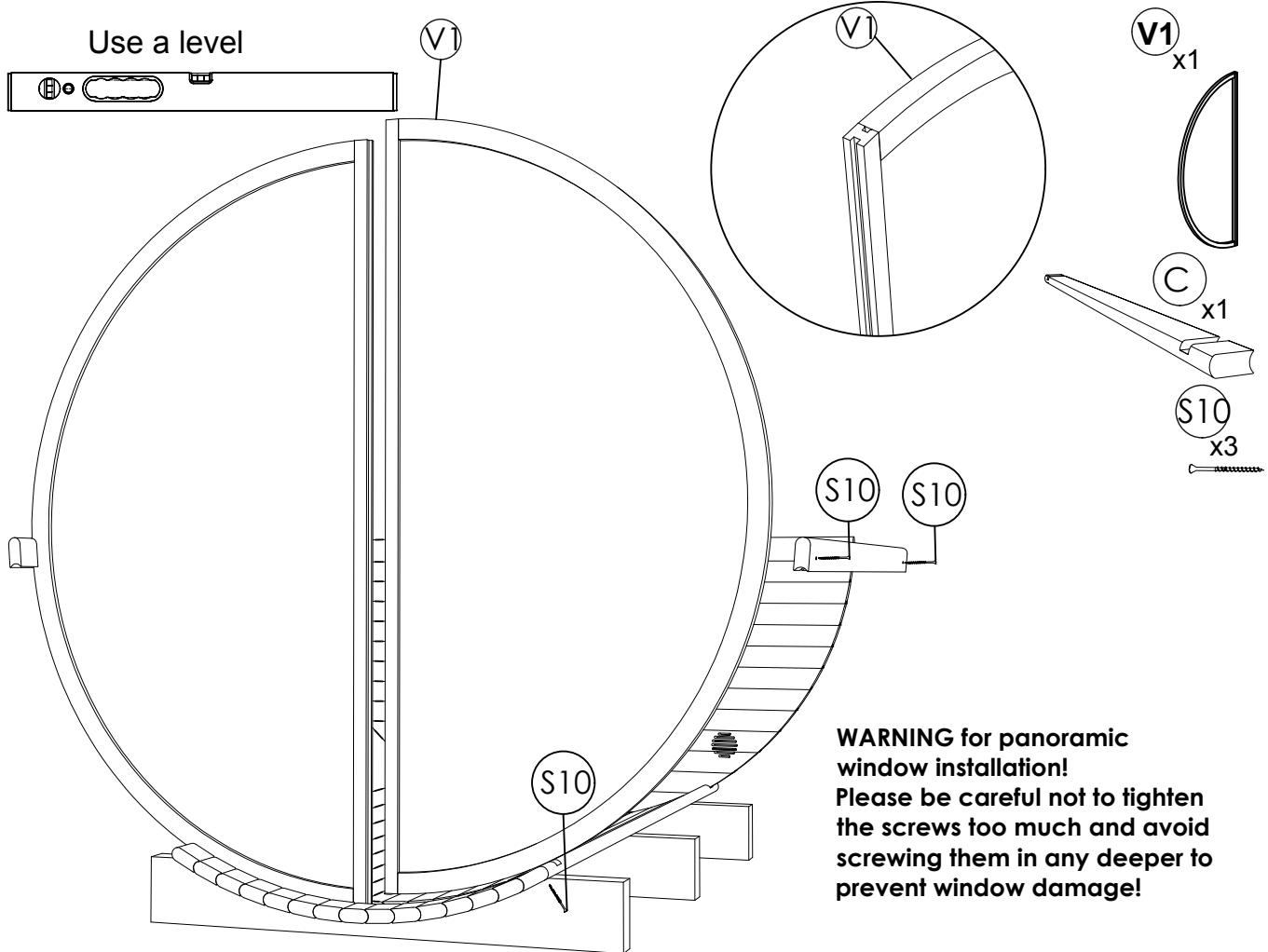
**STEP 3:** Fix Assembly tape with five 4x30 screws (S12) to fix both panels together. Continue placing body staves (C) tightly on both sides of the sauna using rubber mallet, and fixing body staves with screws 4.0x60(S10), two screws for each stave.
