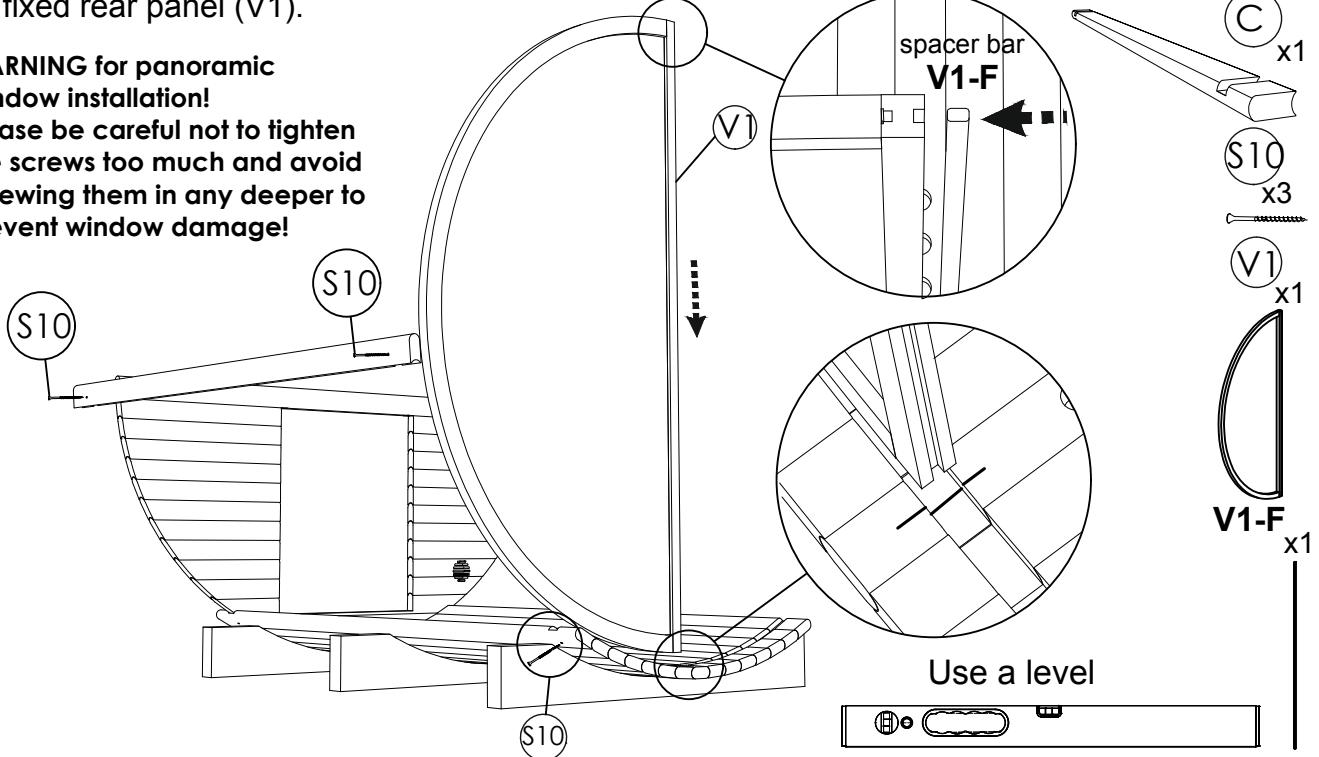
**STEP 2:** Place second rear panel (V1) in stave groove, be sure panel is centered, leveled, completely seated. Fix panel using 4.0 x 60 (S10) screw through last floor stave. Connect the panels (F; V1) together with body stave (C) with 4.0x60 (S10) screw.
