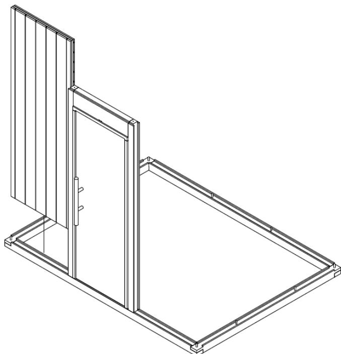
**NOTE:** MAKE SURE TO RUN WIRES UP POSTS AS NEEDED FOR YOUR HEATER OR OTHER ELECTRICAL APPLICATIONS. ALSO MAKE SURE WIRES ARE NOT GETTING PINCHED BY PANELS OR POSTS AS THEY ARE INSTALLED.
