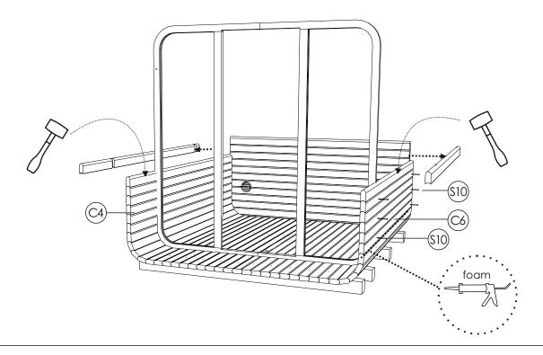
STEP 8: Install the upper rear panelsl (V3;V4) with caution. Use foam between panels for insulation. Place it on top of the back panel. Check that side edges are aligned properly with both panels. One keeps holding the panel in line, and the other is fixing the staves (C; C1) on each sides curve using screws 4x60(S10). Check levels and fix the panel with screws at the ends of the panel's lower sides using screws 5x120(S4).
