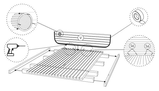
**STEP 4:** Attach adhesive tape along the rear panel (V2)edge. Pre-drill holes then fix panel V2 to panel V with two screws 5x120(S4). Between both panels use foam for better insulation.
