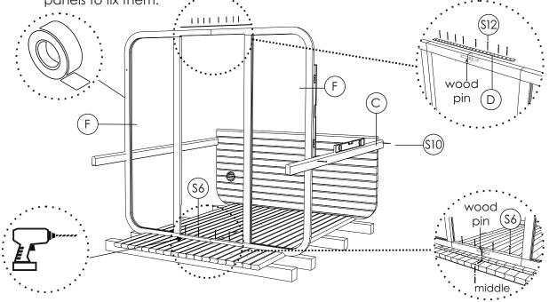
STEP 6: For both sides, the 10th to 11th stave (C) needs to be fixed as one piece. One is holding those three staves, and the other is fixing only the 12th; 13th; 14th; stave with screws 4x60(\$10). Between floor panel and every stave use foam for better insulation.
