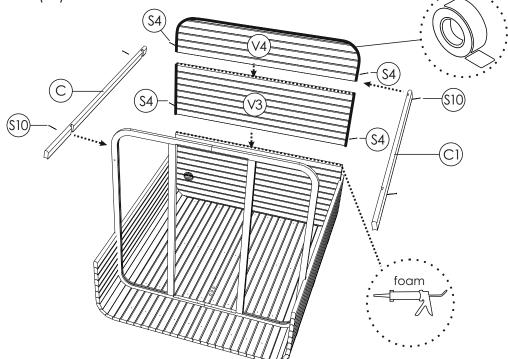
**STEP 9:** Fix the next board panels (C4; C5; C6; C7) on both sides with foam between the stave and panel with screws 4x60(S10) for each side. Use a rubber hammer if necessary, possibly need to push a bit back and front panels.
